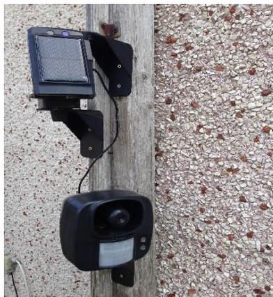
It is pictured here with the optional solar power kit, which means it can be used even in areas that don't have access to mains power. There is also an Ultrasound version which is suitable for noise-sensitive places, such as housing estates.
